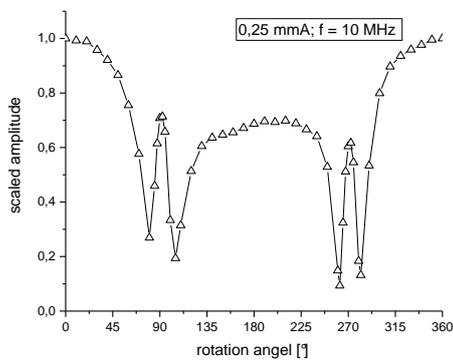
Figure 6: Angle dependent RW pitch catch intensity for borderline crossing.
