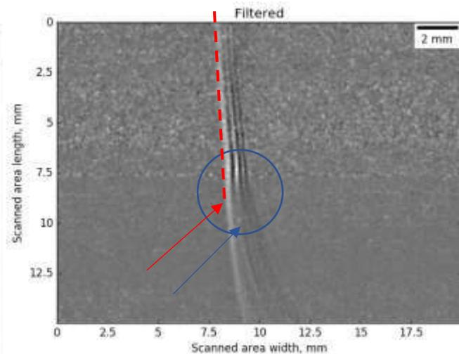
**Figure 4: Snapshot of the Rayleigh wave emitted by a transducer in the peened area (upper part of the image) and orientated by  $\alpha = 6^\circ$  towards the interface.**
