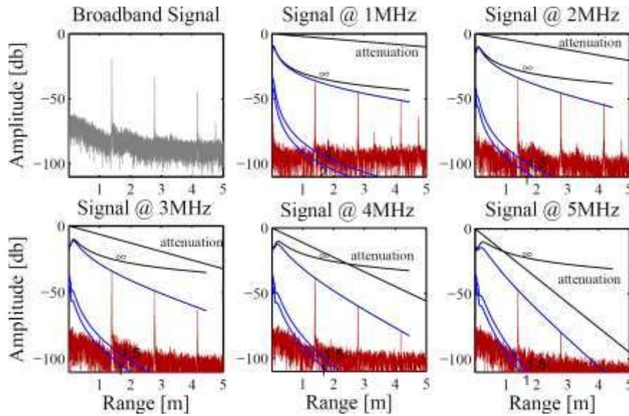
**Figure 2. Example of application of the multi-frequency AVG analysis to data collected with broadband probes centred at 5MHz (Olympus V108 Videoscan). The broadband signal passes to several narrowband filters and the outputs of these filters undergo to a standard single-frequency AVG analysis. The defect detection capability depends on the frequency of the analysis and in this case it is maximum at 3 MHz**
