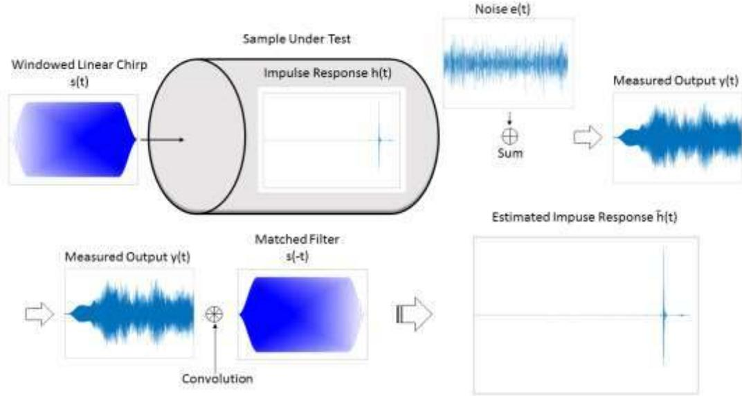
**Figure 1. Block diagram of the PuC measurement procedure implemented. A windowed linear chirp is used as coded excitation signal. The output signal, at which is added an Arbitrary White Gaussian Noise, is then filtered with the matched filter, corresponding in the present case to the time reversed replica of the input signal. After the application of the PuC, an estimate of the impulse response, i.e. the reflectogram, is retrieved.**
