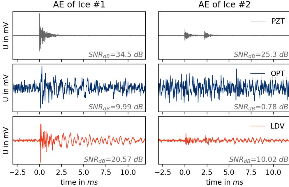
**Figure 4: Two AE signals with different energies emitted by melting ice, detected with three different measurement methods and filtered with analogue and digital filters. (Digital filters: PZT: low-pass 80 kHz, OPT: band-pass 0.5 - 13 kHz, LDV: band-pass 1.5 - 18 kHz)**
