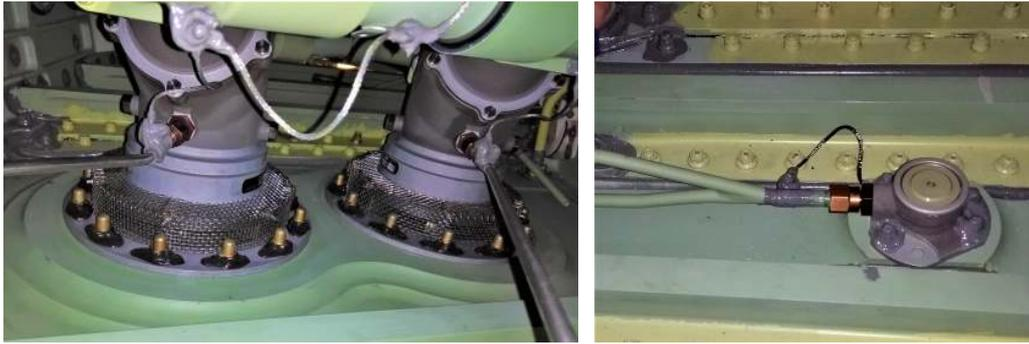
**Figure 1: Left: Fuel pumps 1 and 2 with suction pipes (silver, facing towards viewer) which end at the lowest point of the wing. Right: Drain valve and suction pipe inside an AIRBUS A330 wing tank. The suction pipe connects the drain valve with the lowest point of the tank.**
