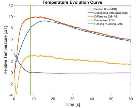
Fig. 4 Temperature evolution curve for perfect bond, artificial debonding with brass, and the difference of two curves. The filtered derivative of artificial debonding with brass inclusion is shown along with heating/cooling gate.
