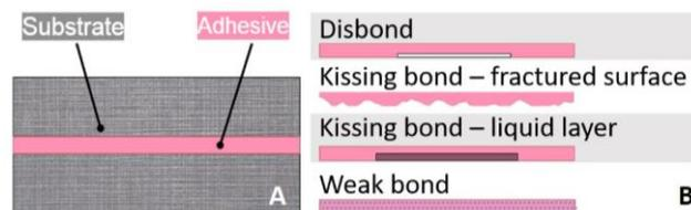
Fig. 1 A) Schematic of adhesive bond adhesive and substrate (adherend) B) Different quality of bonding with interface defect.
