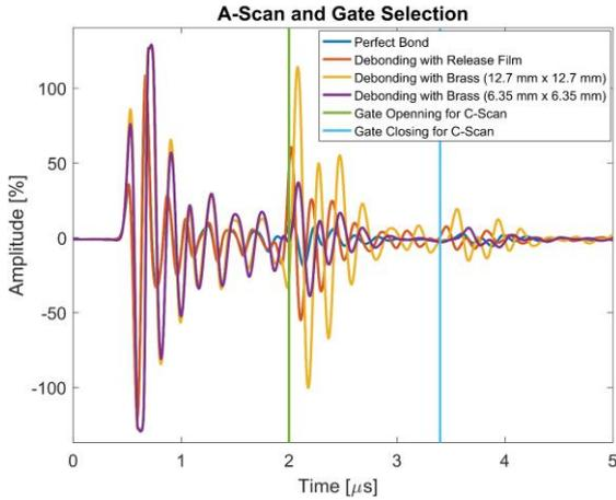
Fig. 3 Ultrasonic inspection A-scan results for perfect bond, artificial debonding with release film, and artificial debonding with brass inclusion with two different size. Gate selection for C-scan image is shown.
