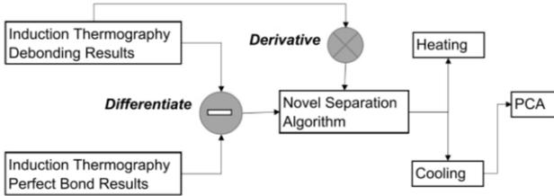
Fig. 6 Schematics of analysis algorithm for induction thermography bonding quality evaluation.
