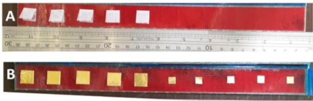
Fig. 2 A) Artificial debonding created by release film inclusion and perfect bond prior to bonding. B) Artificial debonding created by different size brass inclusions prior to bonding.
