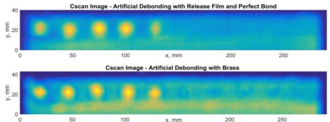
Fig. 5 Ultrasonic inspection C-scan results for artificial debonding with release film, perfect bond, and artificial debonding with brass inclusion. The gate selection has been done according to Fig. 3.
