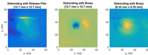
Fig. 7 Principal component analysis of induction thermography results for artificial debonding with release film inclusion and artificial debonding with brass inclusion.
